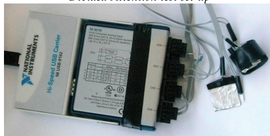
Detail of NI 9219 with sensors
